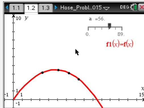
3. a. For the case where  $\theta = 30^\circ$ , find the position of the highest point reached by the jet and the position of the point where the jet strikes the ground, and sketch the graph of the curve traced out by the jet.
