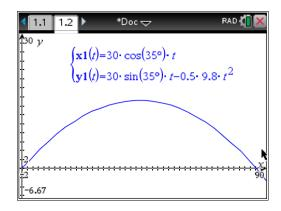
Sketch the graph setting the Window as suggested appropriately. Use Graph Trace to observe the motion of a ball. You can adjust *Tstep* in Window for a more accurate but slower Trace.
